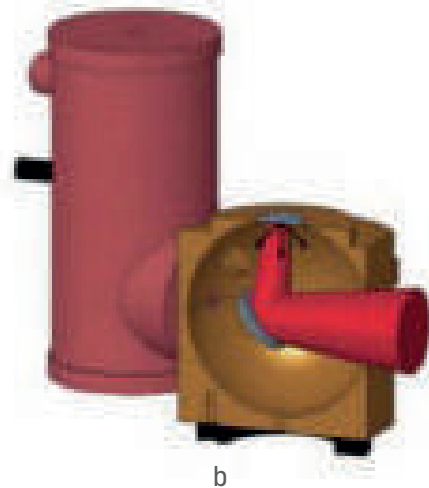
PIKE upward integrated IR gold integrated sphere diagram 5 and 3D drawing.
